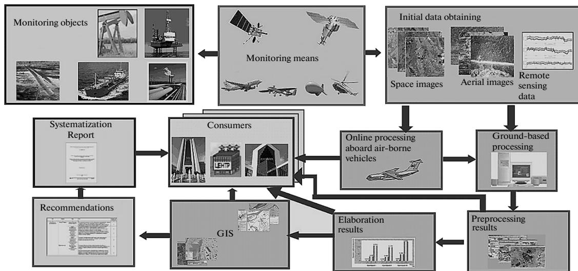
Fig. 2. Schematic diagram of formation of information products during aerospace monitoring of oil and gas areas and facilities.
