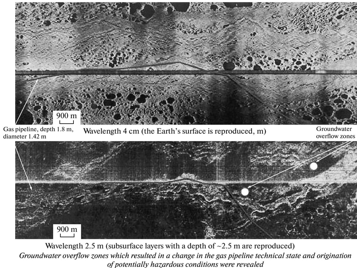
Fig. 7. Multifrequency RIs in the Novyi Urengoi–Surgut gas pipeline segment.
