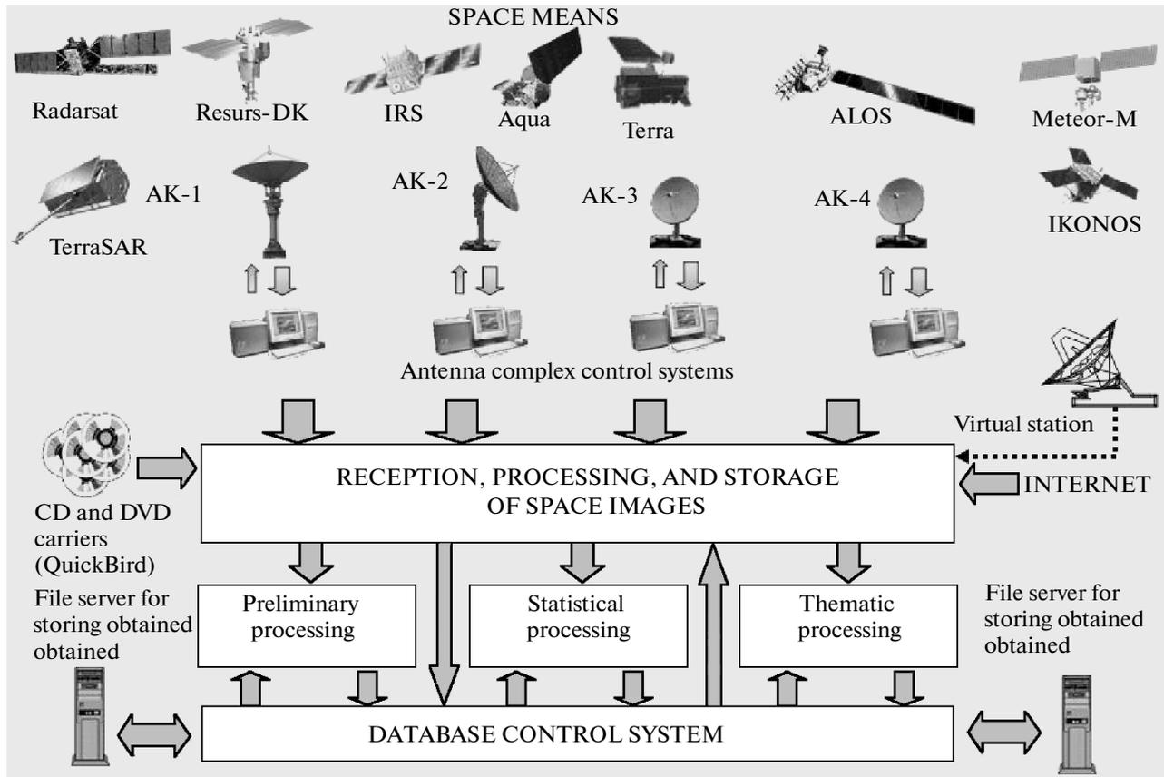
Fig. 3. Organization of data acquisition, processing, and storage during aerospace monitoring.
