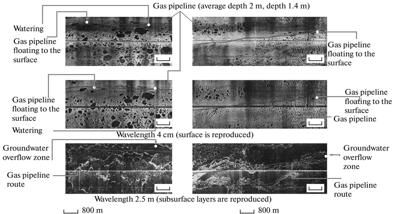
Fig. 8. Multifrequency RIs in segments of the Urengoi–Surgut–Chelyabinsk gas pipeline route.
